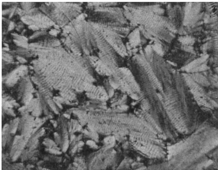
FIGURE 3 The banded focal-conic Fan texture of the chiral smectic C phase Compound 13-6. T = 75^{\circ}\text{C} . ( \times 250 ). Color Plate II, see color plate section.
